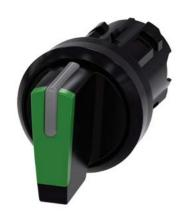
Selector switch, illuminable, 22 mm, round, plastic, green, selector switch, short, 3 switch positions I>O<II, momentary contact on the left, latching on the right, actuating angle  $2x45^{\circ}$ , 10:30h/12h/13:30h, with laser labeling, lower case
