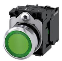
Illuminated pushbutton, 22 mm, round, metal, shiny, green, pushbutton, flat, momentary contact type, with holder, 1NO, LED module with integrated LED 24 V AC/DC, screw terminal, with laser labeling, upper case and lower case, Always upper case at the beginning of the word
