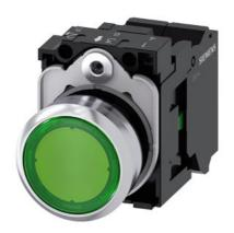
Illuminated pushbutton, 22 mm, round, metal, shiny, green, pushbutton, flat, momentary contact type, with holder, 1NO, LED module with integrated LED 110 V AC, spring-type terminal, Z=20-unit packaging
