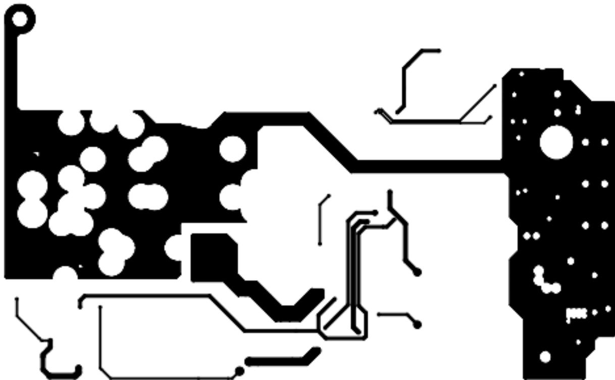
Figure 14-2 Top view of layer 2 (inner signal)
