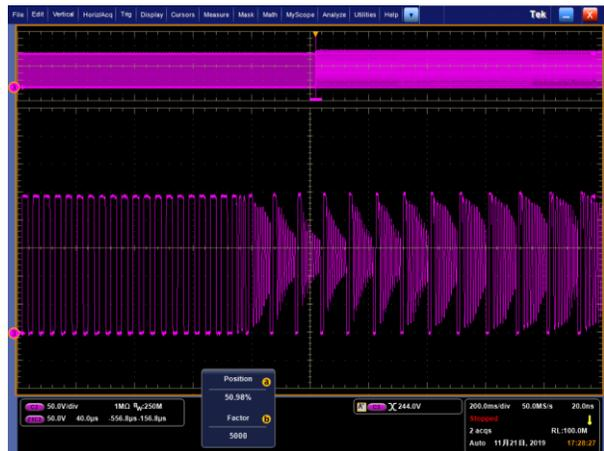
**Figure 9-2** ACF to DCM in 100Vac, V=50V/div, H=40µs/div
