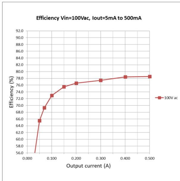
**Figure 12-3** (Detailed) Output current = 5mA to 0.5A
