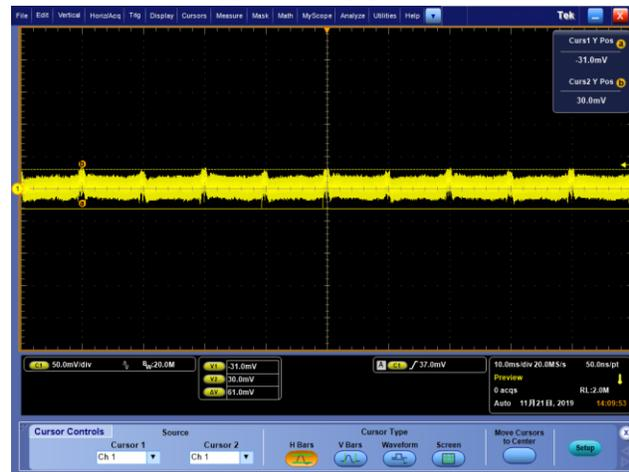
Figure 4-3 Vin=100Vac, V=50mV/div, H=10ms/div
