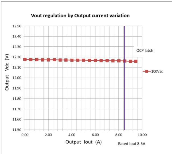
**Figure 11-1** Input voltage=100Vac
