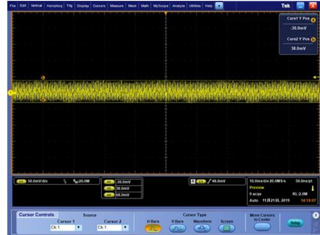
Figure 4-4 Vin=230Vac, V=50mV/div, H=10ms/div
