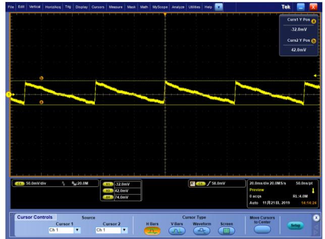
Figure 4-2 Vin=230Vac, V=50mV/div, H=20ms/div
