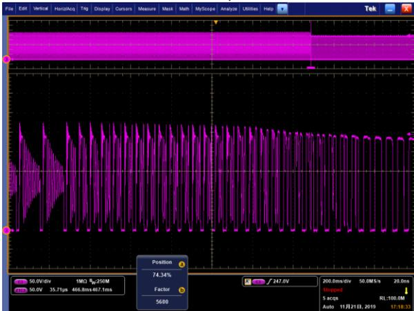
**Figure 9-1** DCM to ACF in 100Vac, V=50V/div, H=35µs/div
