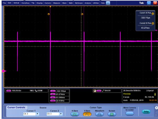
**Figure 8-1** No-load, V=100V/div, H=20ms/div, Skip mode, f=22.9 kHz
