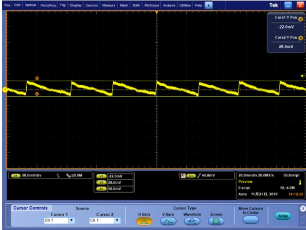
Figure 4-1 Vin=100Vac, V=50mV/div, H=20ms/div
