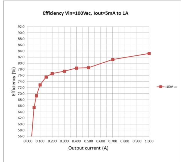
**Figure 12-2** (Detailed) Output current = 5mA to 1A
