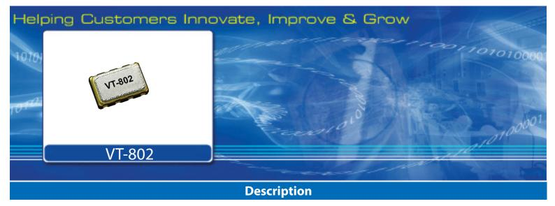
Vectron's VT-802 Temperature Compensated Crystal Oscillator (TCXO) is a quartz stabilized, CMOS output, analog temperature compensated oscillator, operating off either 2.5 or 3.3 volt supply in a hermetically sealed 5.0 x 3.2 ceramic package.
