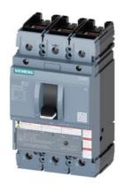
circuit breaker 3VA5 UL frame 250 breaking capacity class C 100kA @ 480 V 3-pole, line protection TM230, FTAM, ln=90A overload protection lr=90A fixed short-circuit protection li=5...10 x ln UL489 SB (naval), 50 deg. cel. cable connection on both sides
