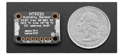
This is where the HTS221 Temperature and Humidity Sensor by ST comes in. With an HTS221, you can take measurements of the relative humidity which will tell you if the environment you're measuring is bone dry or sopping wet. The HTS221 can measure relative humidity from 0%-100% rH with a sensitivity of 0.004% and 3.5% accuracy. It can also measure temperature from -40 to 120 degrees C, with a resolution of 0.016°C with  $\pm$ 0.5 °C accuracy between 15 and +40 °C.
