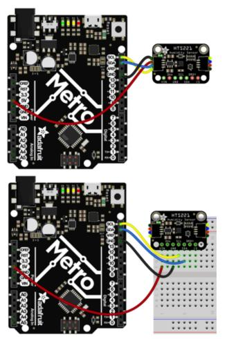
Connect board VIN (red wire) to Arduino 5V if you are running a 5V board Arduino (Uno, etc.). If your board is 3V, connect to that instead. Connect board GND (black wire) to Arduino GND Connect board SCL (yellow wire) to Arduino SCL
