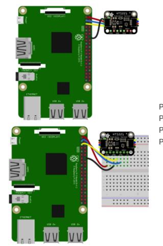
Pi 3V to sensor VCC (red wire) Pi GND to sensor GND (black wire) Pi SCL to sensor SCL (yellow wire) Pi SDA to sensor SDA (blue wire)
