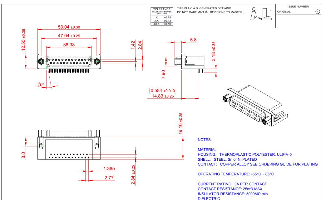
WITHSTANDING VOLTAGE: 1000V AC rms
