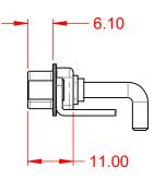
NOTES: MATERIAL: HOUSING: THERMOPLASTIC POLYESTER, UL94V-0 SHELL: STEEL, TIN PLATED CONTACT: COPPER ALLOY, 30µ" GOLD PLATED **OPERATING TEMPERATURE:** -55°C ~ 125°C (CURRENT) PER CONTACT ηΩ ΜΑΧ. Θ 0MΩ min.  $\bigcirc$ 6 0 0  $\cap$
