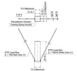
StyleResin CoatedDescriptionResin Coated Type Multilayer Piezoelectric<br/>ActuatorsYoung's<br/>Modulus4.4x10^10 N/m^2RoHSWith ExemptionsSCIP Number294b4799-b00c-43e2-a15f-798c927a3ac8REACHSVHC (PZT - CAS 12626-81-2)
