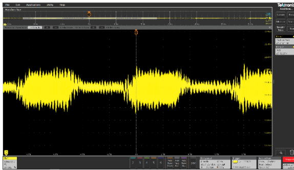
Figure 26. Transient Load on 12 V BUS
