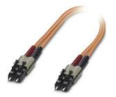
Assembled FO cable, zip cord cable, multi-mode fiberglass 50/125  $\mu$ m, OM2, plug: LC/LC, degree of protection: IP20, for installation in cable ducts or control cabinets, length: 1 m
