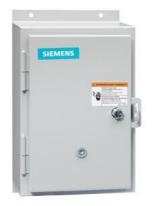
Non-reversing motor starter, Size 1 3/4, Three phase full voltage, Solidstate overload relay, OLR amp range 10-40A, Non-combination type, Enclosure type 12, Dust/drip proof for indoors, Extra-wide enclosure
