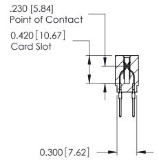
725 Series Ultra-Mate Card Edge Connector - Press Fit Part Number: 725-074-522-201 **EDAC INC** THESE DRAWINGS AND SPECIFICATIONS ARE THE PROPERTY OF EDAC INC.,AND TORONTO, ONTARIO SHALL NOT BE REPRODUCED, OR COPIED CANADA
