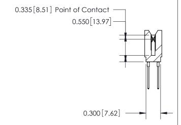
745 Series Ultra-Mate Card Edge Connector - Press Fit Part Number: 745-052-545-206 **EDAC INC** THESE DRAWINGS AND SPECIFICATIONS ARE THE PROPERTY OF EDAC INC.,AND TORONTO, ONTARIO SHALL NOT BE REPRODUCED, OR COPIED CANADA OR USED AS THE BASIS FOR THE MANUFACTURE OR SALE OF APPARATUS YOUR CONNECTION TO QUALITY & SERVICE WITHOUT WRITTEN PERMISSION.
