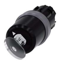
Key-operated switch BKS, 22 mm, round, plastic with metal front ring, lock number S1, with 2 keys, 2 switch positions O<I, momentary contact type, Actuating angle  $45^{\circ}$ , 10:30h/12h, key removal O, with laser labeling, lower case
