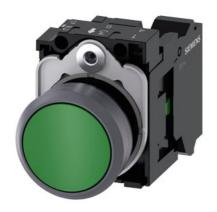
Pushbutton, 22 mm, round, plastic with metal front ring, green, pushbutton, flat, momentary contact type, with holder, 1 NO, spring-type terminal, Z=20-unit packaging
