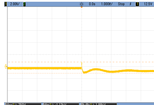
Output voltage waveform (0.75KV)
