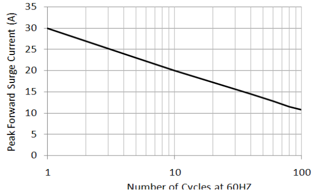
Figure 2. Maximum Non-repetitive Peak Forward Surge Current
