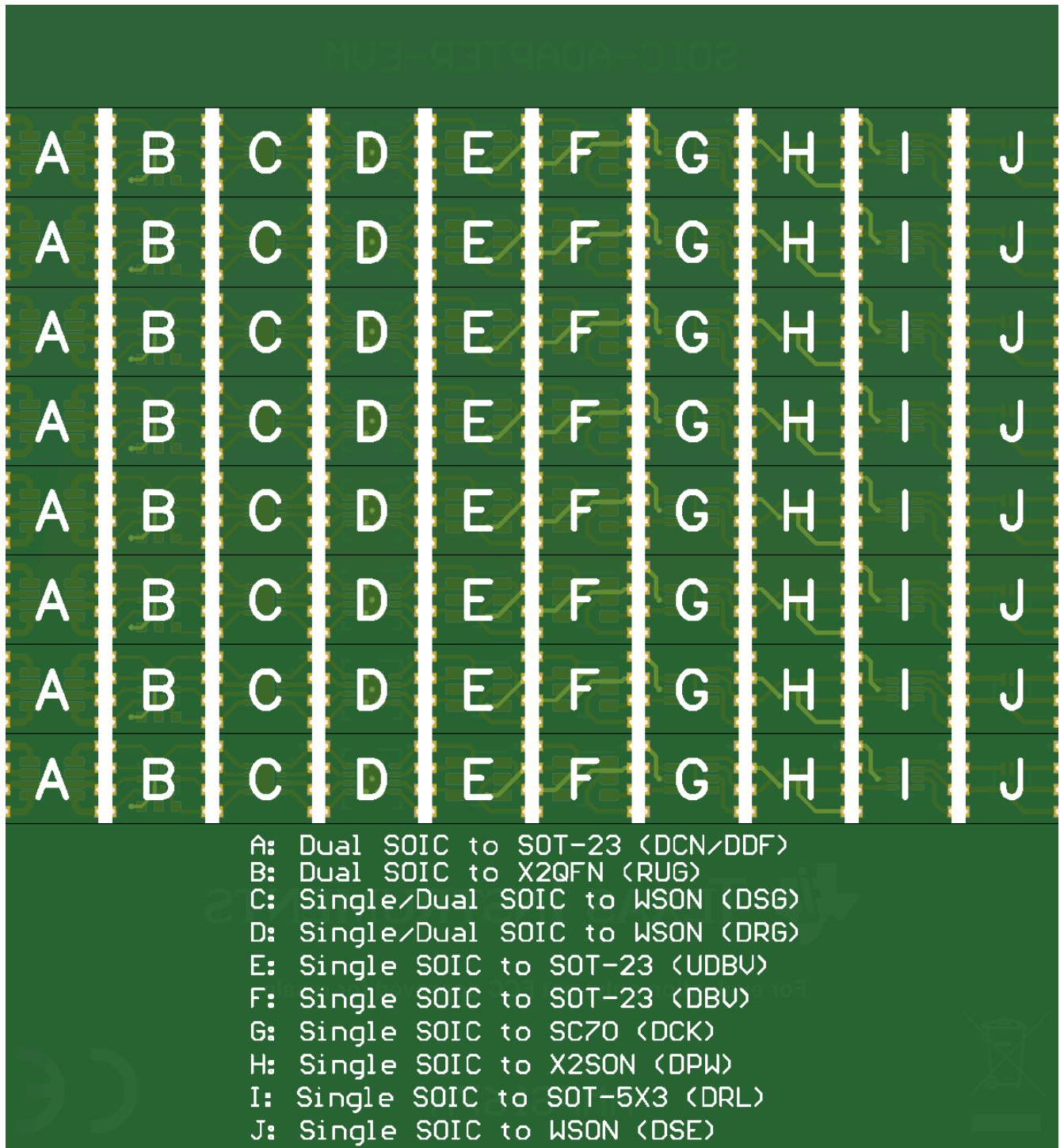
Figure 4-2. PCB Bottom Layer
