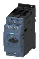
Circuit breaker size S2 for motor protection, CLASS 10 A-release 9.5...14 A N-release 208 A screw terminal Standard switching capacity with transverse auxiliary switches 1 NO+1 NC
