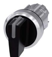
Illuminable selector switch, 22 mm, round, metal shiny, black, Selector switch short, 3 switch positions I-O-II, latching, actuating angle 2x45°, 10:30h/12h/13:30h
