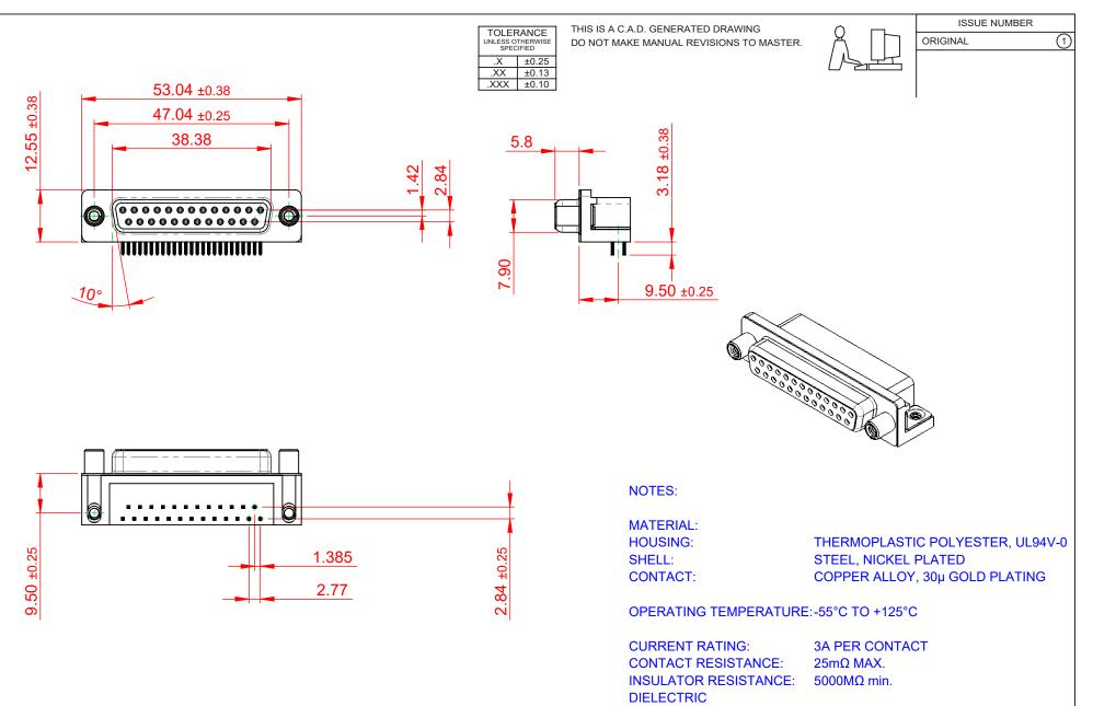
WITHSTANDING VOLTAGE: 1000V AC rms
