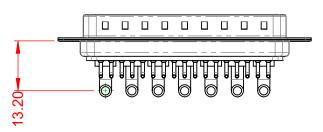
POWER/CO-AX CONTACT RATING: (IF PRESENT) SIGNAL CONTACT CURRENT RATING: 5A PER CONTACT SIGNAL CONTACT RESISTANCE:  $10m\Omega$  MAX. INSULATOR RESISTANCE: 5000MΩ min.
