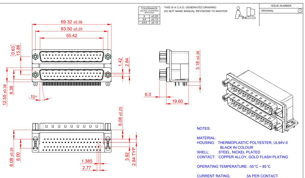
CONTACT RESISTANCE:  $25m\Omega$  MAX. INSULATOR RESISTANCE:  $5000M\Omega$  min. DIELECTRIC WITHSTANDING VOLTAGE: 1000V AC rms
