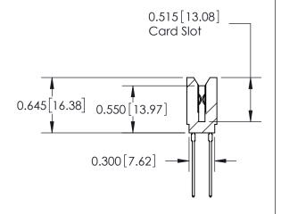
ACAD REFERENCE NO. 737 Series Ultra-Mate Card Edge Connector - Press Fit DRAWN: Part Number: 737-018-541-206 CHECKED: **EDAC INC** SCALE: THESE DRAWINGS AND SPECIFICATIONS ARE THE PROPERTY OF EDAC INC.,AND TORONTO, ONTARIO SHALL NOT BE REPRODUCED, OR COPIED DRAWING NUMBER CANADA OR USED AS THE BASIS FOR THE 737-ENG MASTER MANUFACTURE OR SALE OF APPARATUS YOUR CONNECTION TO QUALITY & SERVICE WITHOUT WRITTEN PERMISSION.
