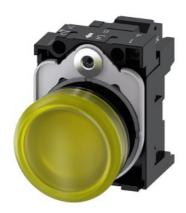
Indicator lights, 22 mm, round, plastic, yellow, lens, smooth, with holder, LED module, with integrated LED 24 V AC/DC, spring-type terminal, with laser labeling, lower case
