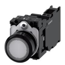
Illuminated pushbutton, 22 mm, round, plastic, clear, pushbutton, flat, momentary contact type, with holder, 1 NO+1 NC, LED module with integrated LED 110 V AC, spring-type terminal, with laser labeling, upper case and lower case, always upper case at beginning of line
