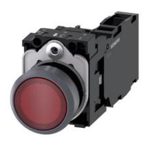
Illuminated pushbutton, 22 mm, round, plastic with metal front ring, red, pushbutton, flat, momentary contact type, with holder, 1 NO+1 NC, LED module with integrated LED 110 V AC, screw terminal, with laser labeling, upper case and lower case, Always upper case at the beginning of the word
