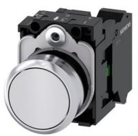
Pushbutton, 22 mm, round, metal, shiny, white, pushbutton, flat, momentary contact type, with holder, 1 NO, spring-type terminal, with laser labeling, symbol number according to, ISO 7000 or IEC 60417
