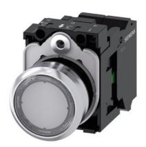
Illuminated pushbutton, 22 mm, round, Metal, shiny, transparent, pushbutton, flat, momentary contact type, with holder, 1NO, LED module with integrated LED 230 V AC, spring-type terminal, with laser labeling, upper case
