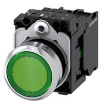
Illuminated pushbutton, 22 mm, round, Metal, shiny, green, pushbutton, flat, momentary contact type, with holder, 1NO, LED module with integrated LED 230 V AC, screw terminal, with laser labeling, upper case and lower case, always upper case at beginning of line
