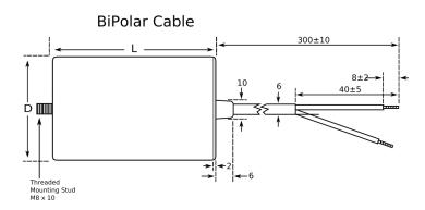
Series C27 Dielectric Film/Foil Polypropylene Style Plastic Case and Cover, Ultra Sonically Welded Description Ultra Sonically Welded Seal, Safety Class PO, **Features** UL 94 V0 Disk RoHS Yes Termination Tin Copper Lead BiPolar Cables UL, VDE, UL (Construction Only), UL\_94 VO Disk Qualifications AEC-Q200 Component 137.2 g Weight
