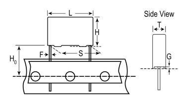
General Information Series F861 Dielectric Metallized Polypropylene Style Radial Features MKP EMI Safety RoHS Lead Wire Leads Safety Class X2 Qualifications ENEC, UL, cUL, CQC AEC-Q200 No THB Performance No 1.566 g Component Weight Miscellaneous ClimCat: 40/110/56/B Shelf Life 104 Weeks
