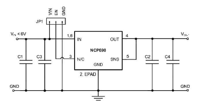
NCP690, 1A, Fixed Output Voltage LDO Schematic View
