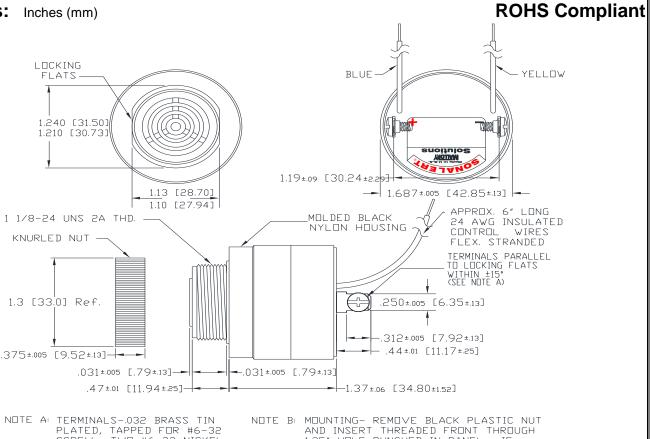
PLATED, TAPPED FOR #6-32 SCREW. TWO #6-32 NICKEL PLATED BRASS SCREWS INCLUDED. WILL ACCEPT 1/4" QUICK CONNECT. NOTE B: MOUNTING- REMOVE BLACK PLASTIC NUT AND INSERT THREADED FRONT THROUGH 1.25" HOLE PUNCHED IN PANEL, IF ORIENTATION IS NEEDD, NOTE LOCKING FLATS ON DRAWING. SCREW NUT BACK ON. DO NOT OVERTIGHTEN.
