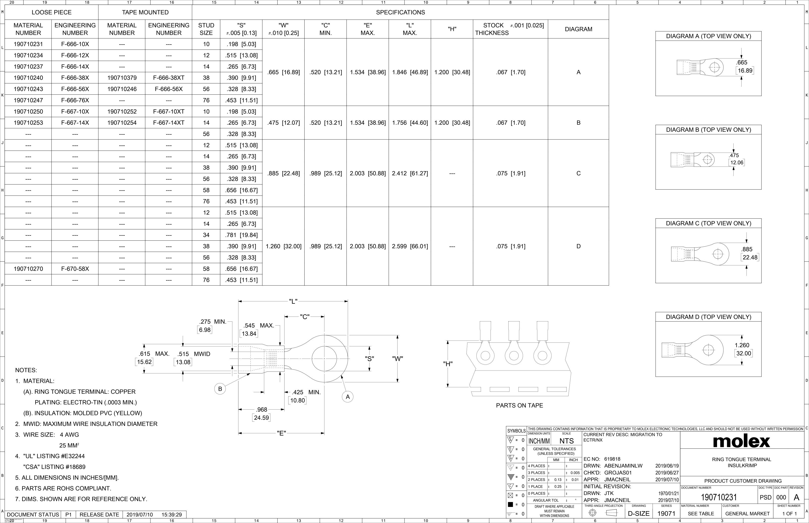
MATERIAL: Copper PLATING: Electro-Tin (.0003 Min.) INSULATION: PVC Color Coded Yellow STUD SIZES: ("D" ±.005) 10 - .198 14 - .265 56 - .328 38 - .39076 - .453 12 - .515 58 - .656 34 - .781 ASSEMBLY IS ROHS COMPLIANT.
