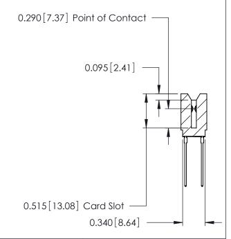
746 Series Ultra-Mate Card Edge Connector - Press Fit Part Number: 746-050-541-206
