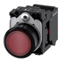
Illuminated pushbutton, 22 mm, round, plastic, red, pushbutton, flat, momentary contact type, with holder, 1NC, LED module with integrated LED 230 V AC, spring-type terminal, with laser labeling, symbol number according to, ISO 7000 or IEC 60417
