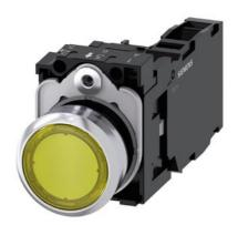
Illuminated pushbutton, 22 mm, round, metal, shiny, yellow, pushbutton, flat, momentary contact type, with holder, 1 NO+1 NC, LED module with integrated LED 24 V AC/DC, screw terminal, Z=20-unit packaging
