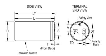
General Information Series ALS40 Dielectric Aluminum Electrolytic Description Screw Terminal, Aluminum Electrolytic RoHS AEC-Q200 No Halogen Free No Component 300 g Weight Dimensions D And L Include Sleeving. MS (MxH) = Notes M12x16. Mounting Clamp (Sold Separately): V4/2737 Shelf Life 156 Weeks
