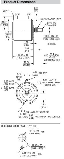
$\frac{2.46}{(.097)}$ RECOMMENDED PCB THICKNESS: MOUNTING TORQUE: 15-18 LB.-IN.
