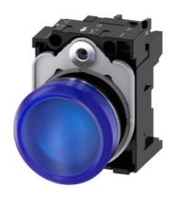
Indicator lights, 22 mm, round, Metal, shiny, blue, lens, smooth, with holder, LED module with integrated LED 230 V AC, screw terminal, with laser labeling, upper case and lower case, always upper case at beginning of line
