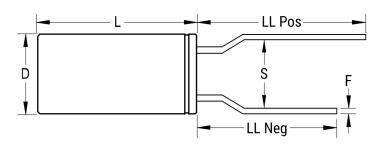
General InformationSeriesESKDielectricAluminum ElectrolyticDescriptionSingle Ended, Aluminum ElectrolyticRoHSYesLeadFormed To 5mmAEC-Q200No
