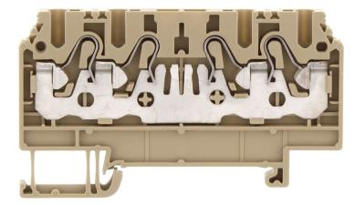
Feed-through terminal, Push-in connection, Mounting type: Mounting rail TS 35/7.5, Rated cross-section: 1.5 mm<sup>2</sup>, Width: 4.1 mm, Colour: Beige
