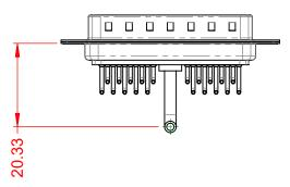
20A (CURRENT) POWER/CO-AX CONTACT RATING: (IF PRESENT) SIGNAL CONTACT CURRENT RATING: 5A PER CONTACT SIGNAL CONTACT RESISTANCE:  $10m\Omega$  MAX. INSULATOR RESISTANCE: 5000MΩ min.
