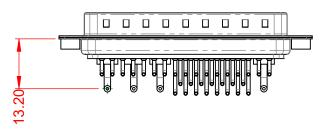
10A (CURRENT) POWER/CO-AX CONTACT RATING: (IF PRESENT) SIGNAL CONTACT CURRENT RATING: 5A PER CONTACT SIGNAL CONTACT RESISTANCE:  $10m\Omega$  MAX. INSULATOR RESISTANCE: 5000MΩ min. DIELECTRIC
