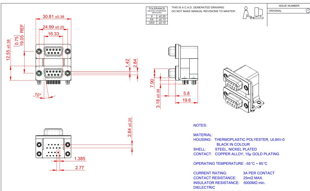
WITHSTANDING VOLTAGE: 1000V AC rms
