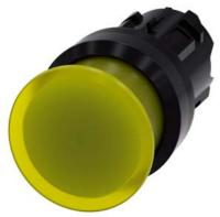
Illuminated mushroom pushbutton, 22 mm, round, plastic, yellow, 30 mm, momentary contact type, with laser labeling, upper case and lower case, always upper case at the beginning of the word
