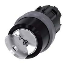
RONIS key-operated switch, 22 mm, round, plastic with metal front ring, lock number SB30, with 2 keys, 2 switch positions O-I, latching, actuating angle 90°, 10:30h/13:30h, key removal O+I, possible special locks: SB31, 421, 455 Z=50-unit packaging
